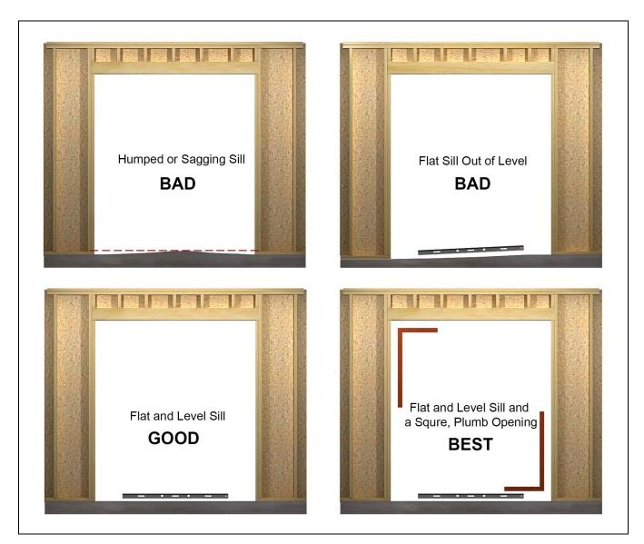
The key to proper operation is squaring the frame in relation to the sill. A GOOD installation has a FLAT sill that is also LEVEL The BEST INSTALLATION requires a FLAT and LEVEL sill and a SQUARE and PLUMB opening
