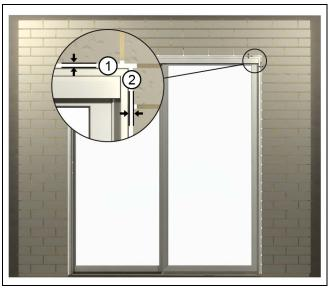
Figure 2 Masonry opening clearance
