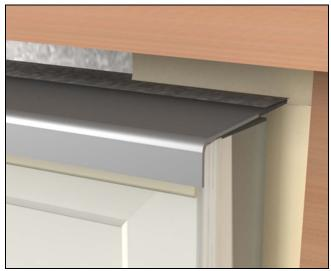
Figure 30 Apply sealant between window and exterior finish at head jamb.
